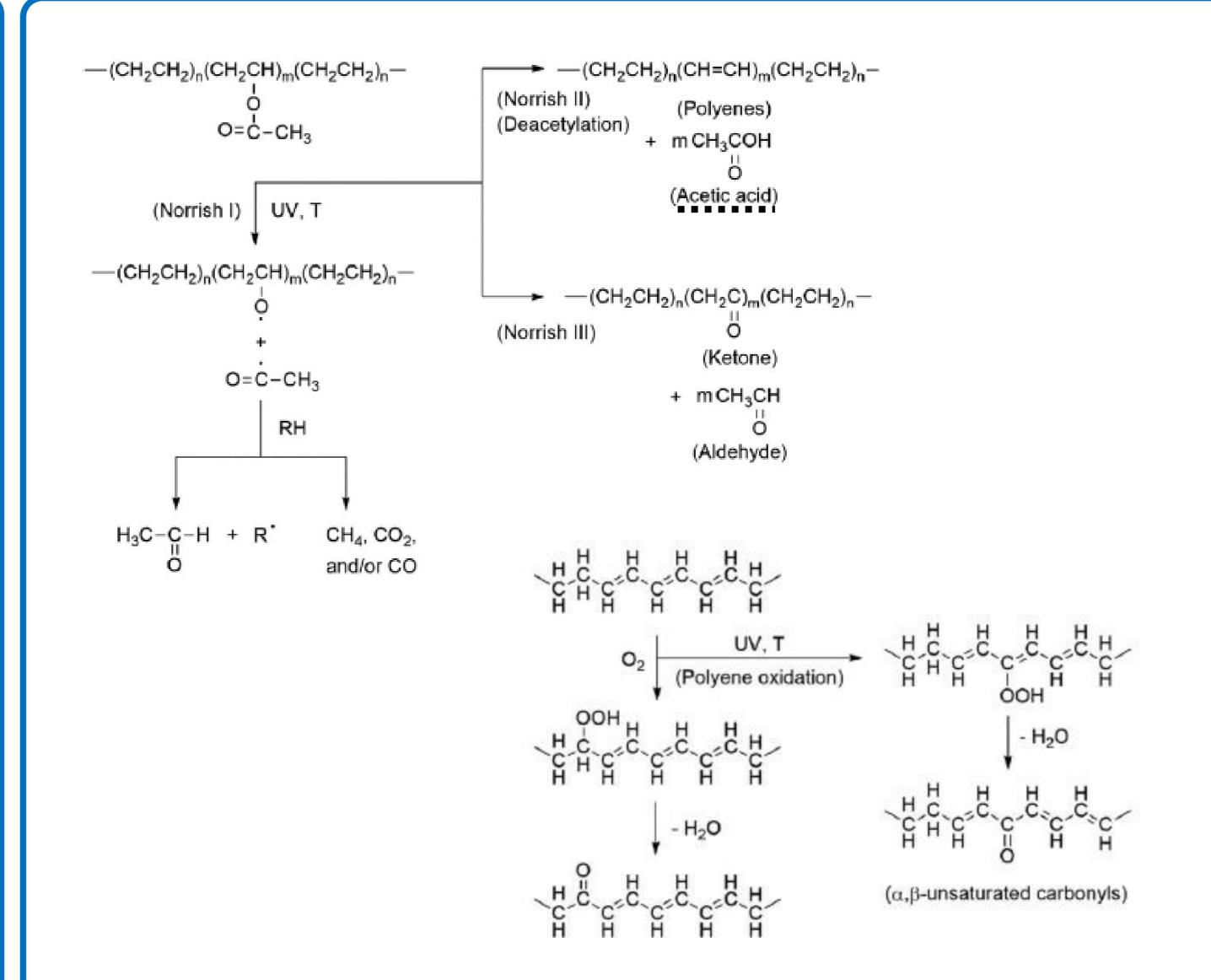
Photo-oxidative reactions produce acetic, which works as a catalyst for deacetylation reactions and further degradations. Yellowing of EVA can also occur during aging and it is due to the interactions between encapsulants additives and products of the photooxidation reactions.
