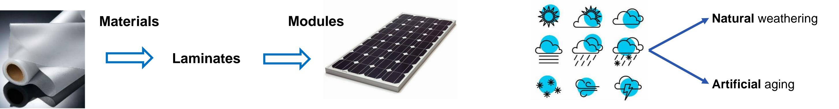
In order to determine characteristics of material interactions and the exact reaction patways occurring during aging different levels will be investigated: materials, laminates and PV modules. The influence of different climatic conditions on reaction kinetics will be analysed and samples will be subjected to natural weathering and artificial aging.
